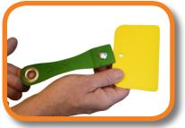
• For quick change of spreaders for cleaning, insert spreader in front of bolt and tighten.
