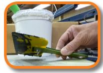
• The wing nut doubles as "feet" to keep the spreader angled up, off of surfaces and easy to pick up!
