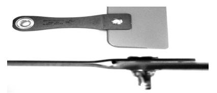
To quick change spreaders for cleaning, insert spreader in *front* of bolt and tighten wing nut.
